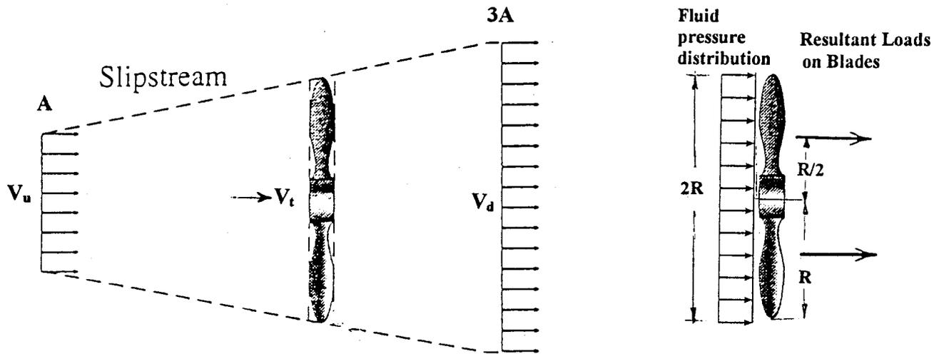
Optimal conditions:  $A_d = 3A$ ,  $V_d = 1/2V_t$ , Efficiency = 59.3%
