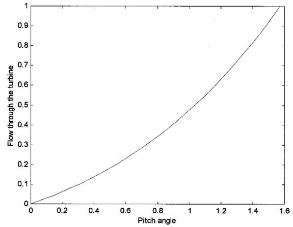
**Fig. 7 Flow through  $s$  versus pitch angle  $\varphi$**
