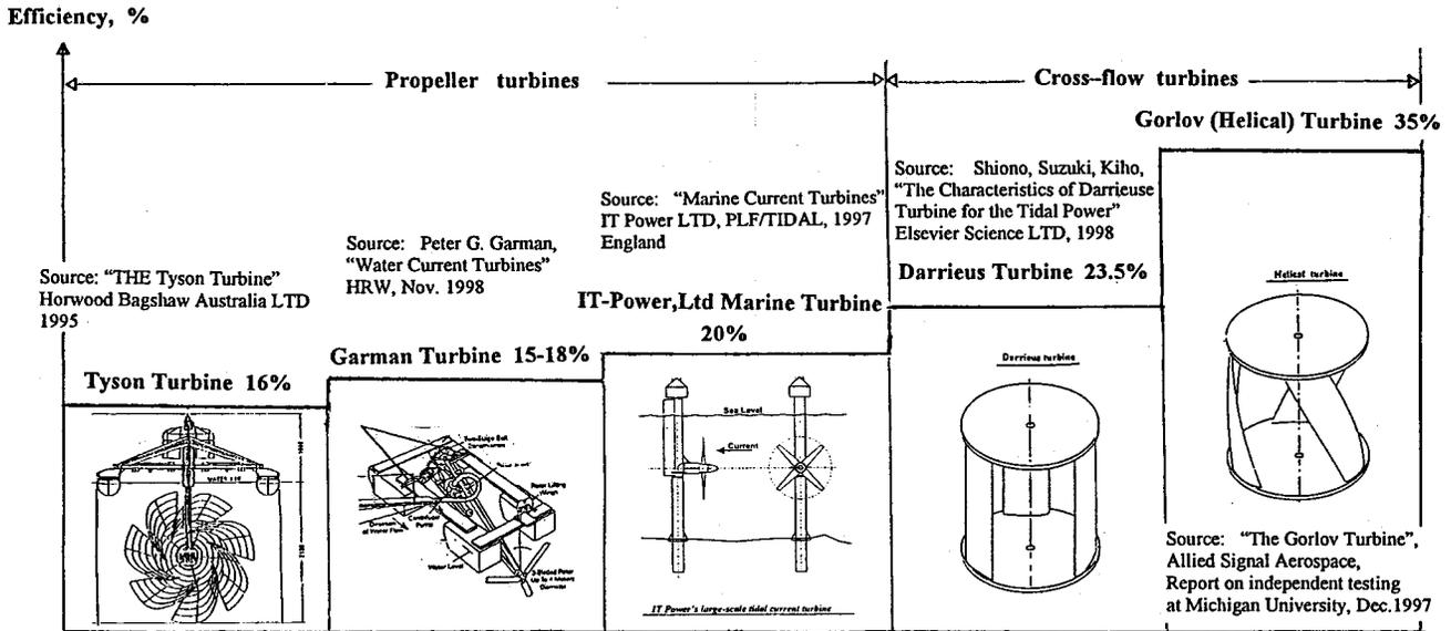
Note: Some specific exploitation problems for Propeller and Darrieus turbines
