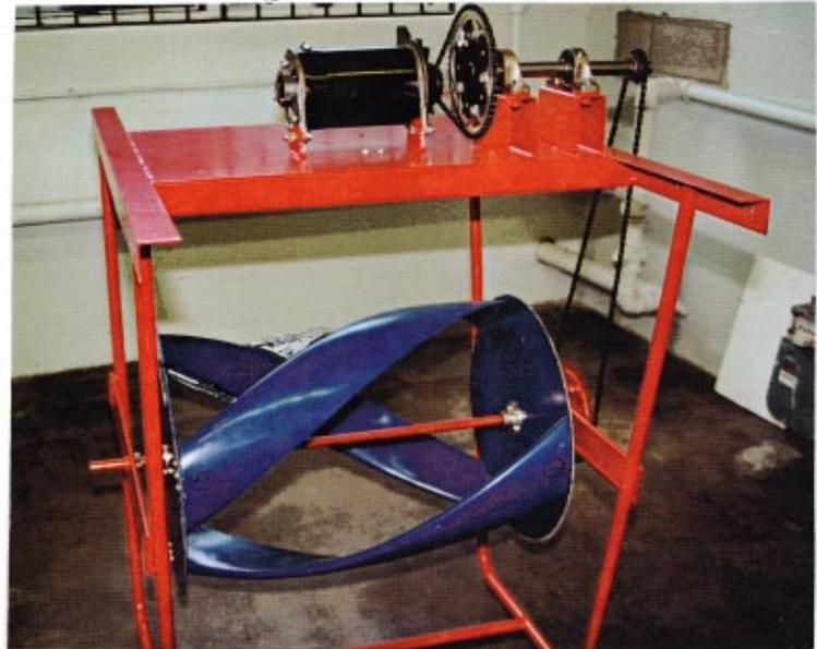
Fig. 3 Power systems for free flows with different helical turbines
