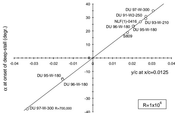
**Figure 23: Correlation of deep-stall angle with leading edge thickness for a number of wind turbine airfoils**
