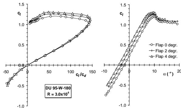
**Figure 8: The effect of a flap deflection on the performance of DU 95-W-180 at  $R=3 \times 10^6$ .**
