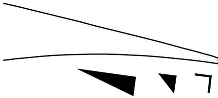
**Figure 17: Sketch of the Gurney flap and some wedges applied to the trailing edge of DU 93-W-210**
