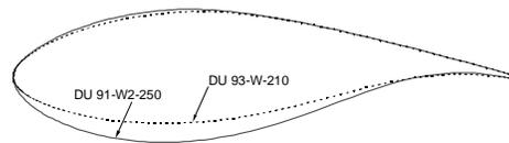
Figure 6: The airfoil shapes of DU 91-W2-250 and DU 93-W-210
