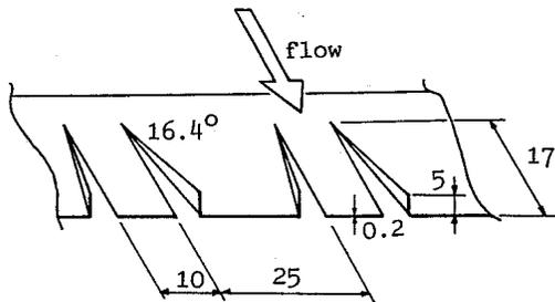
**Figure 20: Sketch of the vortex generators used during most wind tunnel tests. Dimensions in mm**
