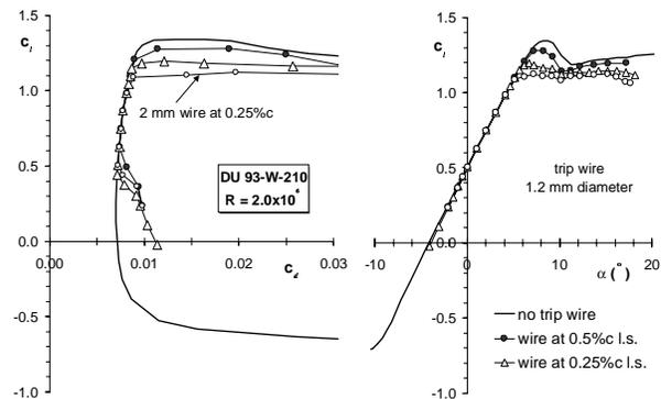
**Figure 19: The effect on performance of thickness and location of a trip wire located on the leading edge of DU 93-W-210**
