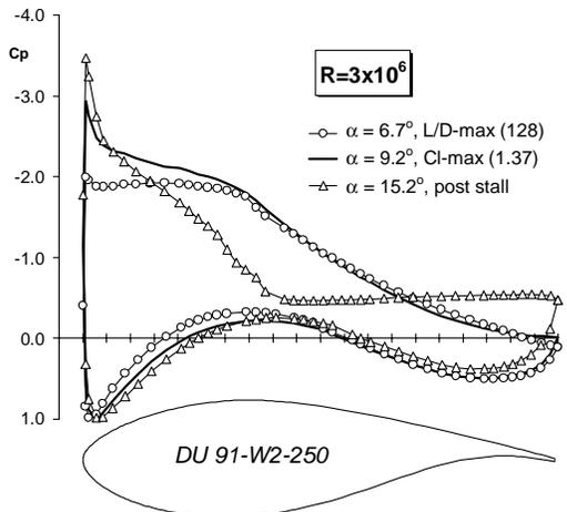
Figure 4: Measured pressure distributions for DU 91-W2-25 at  $R=3 \times 10^6$
