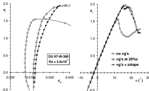
**Figure 21: effect of vortex generators on the performance of DU 97-W-300 with and without zigzag tape**
