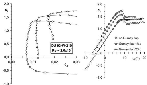
**Figure 16: The effect of 1% $c$  and 2% $c$  Gurney flaps on the performance of DU 93-W-210.**
