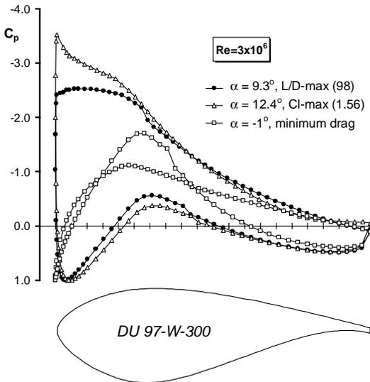
**Figure 12: Measured pressure distributions for airfoil DU 97-W-300 at  $R=3 \times 10^6$**
