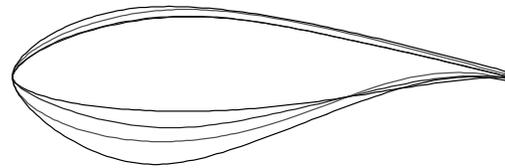
**Figure 1: A series of DU airfoils for a pitch regulated 55 m diameter rotor.**
