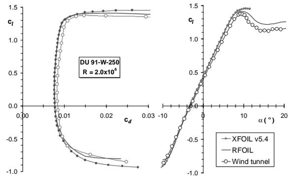
**Figure 3: The prediction of DU 91-W2-250 characteristics with XFOIL and RFOIL**
