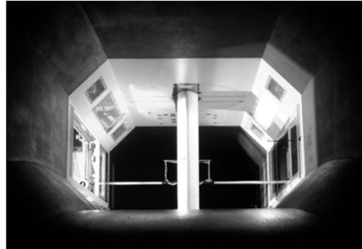
**Figure 2: The model of airfoil DU 97-W-300 in the LST test section seen from inside the contraction. The wake rake is in the back.**
