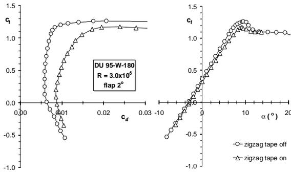
**Figure 10: The effect of zigzag tape at  $x/c=0.05$  on the performance of DU 96-W-180.**
