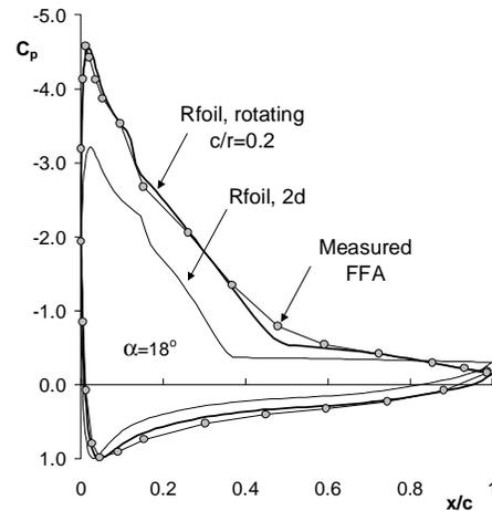
**Figure 11: The predicted and measured effect of rotation on the pressure distribution of the 30% span section of a rotating blade**
