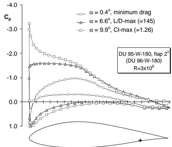
**Figure 9: Measured pressure distributions of airfoil DU 96-W-180 at  $R=3 \times 10^6$ .**
