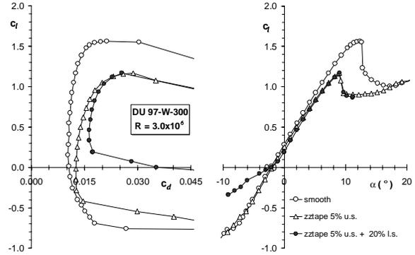
**Figure 13: The effect of zigzag tape on the characteristics of DU 97-W-300 at  $R=3 \times 10^6$**
