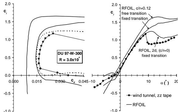
**Figure 15: The RFOIL predicted effect of rotation on DU 97-W-300 in the transition free and fixed condition.**
