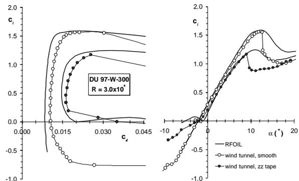
**Figure 14: The measured and calculated performance of DU 97-W-300 at  $R=3 \times 10^6$ .**
