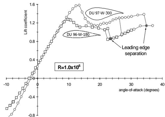
**Figure 22: The lift curves of two DU airfoils showing leading edge separation**
