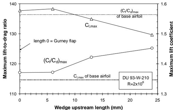
**Figure 18: The effect of wedge upstream length on the  $(l/d)_{max}$  and  $C_{l,max}$  of DU 93-W-210.**
