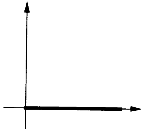
Fig. 3 Force vs. displacement of R23 element
