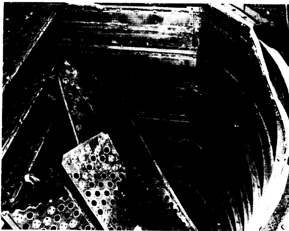
Figure 21: Tray Damage Due to Flashing in the Base of a Column (10 ft. diameter)
