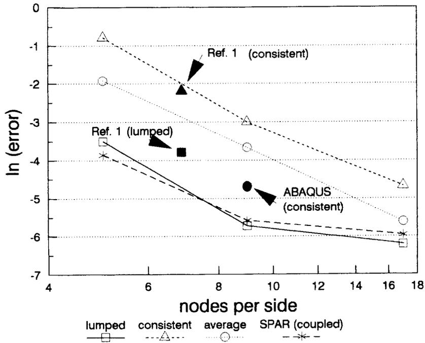
Figure 6. Frequency convergence for mode  $n=4$ ,  $m=1$  of a cylindrical shell as a function of mesh density for different finite elements.
