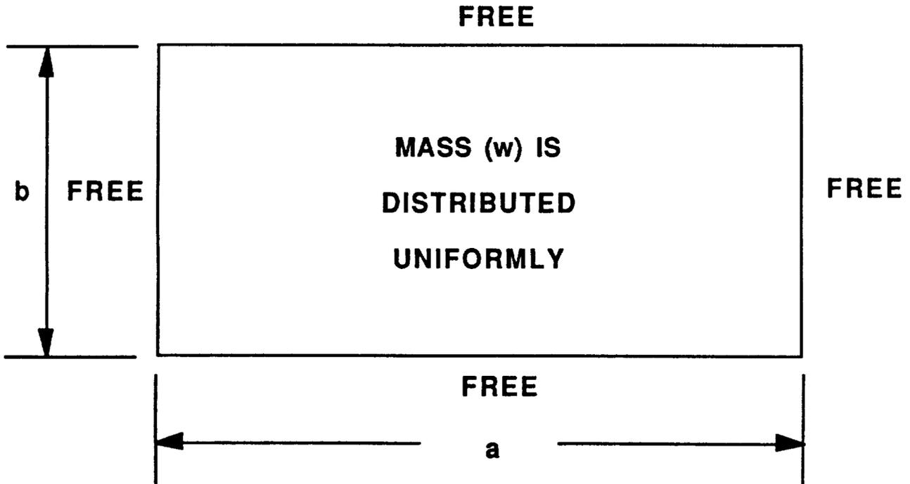
Figure 9. Rectangular Plate Free on All Sides (Example 6)
