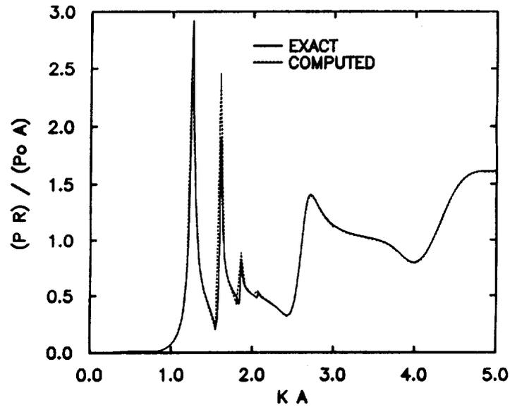
Fig. 3. Forward Scattering from a Fluid-Filled Spherical Shell
