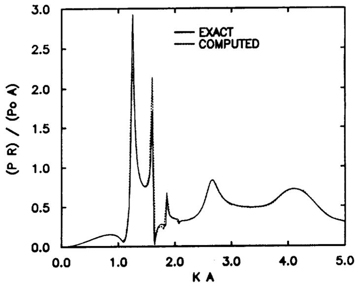
Fig. 4. Backward Scattering from a Fluid-Filled Spherical Shell
