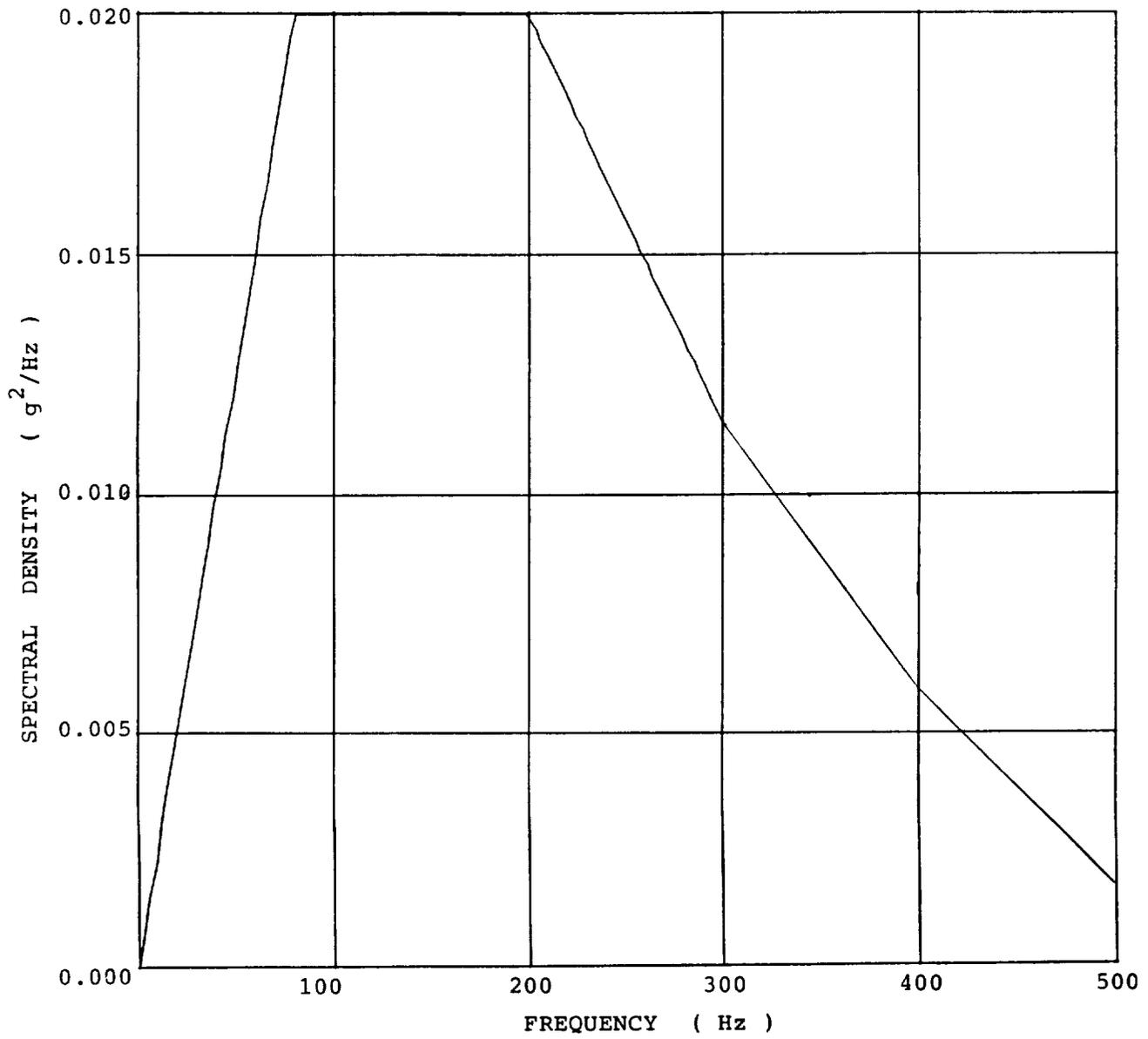
FIG. 3. INPUT ACCELERATION SPECTRUM
