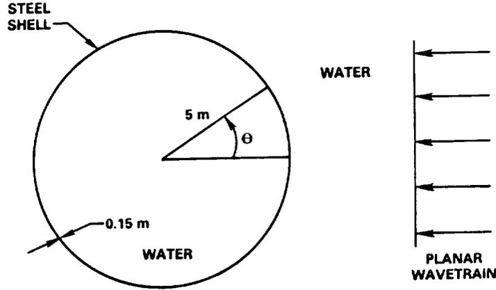
Fig. 2. Plane Wave Scattering from a Fluid-Filled Spherical Shell
