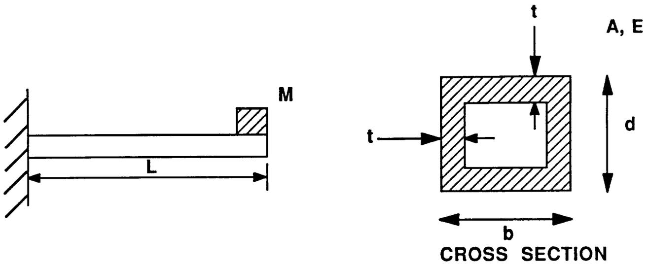
Figure 6. Cantilever Beam with Concentrated Mass (Example 3)
