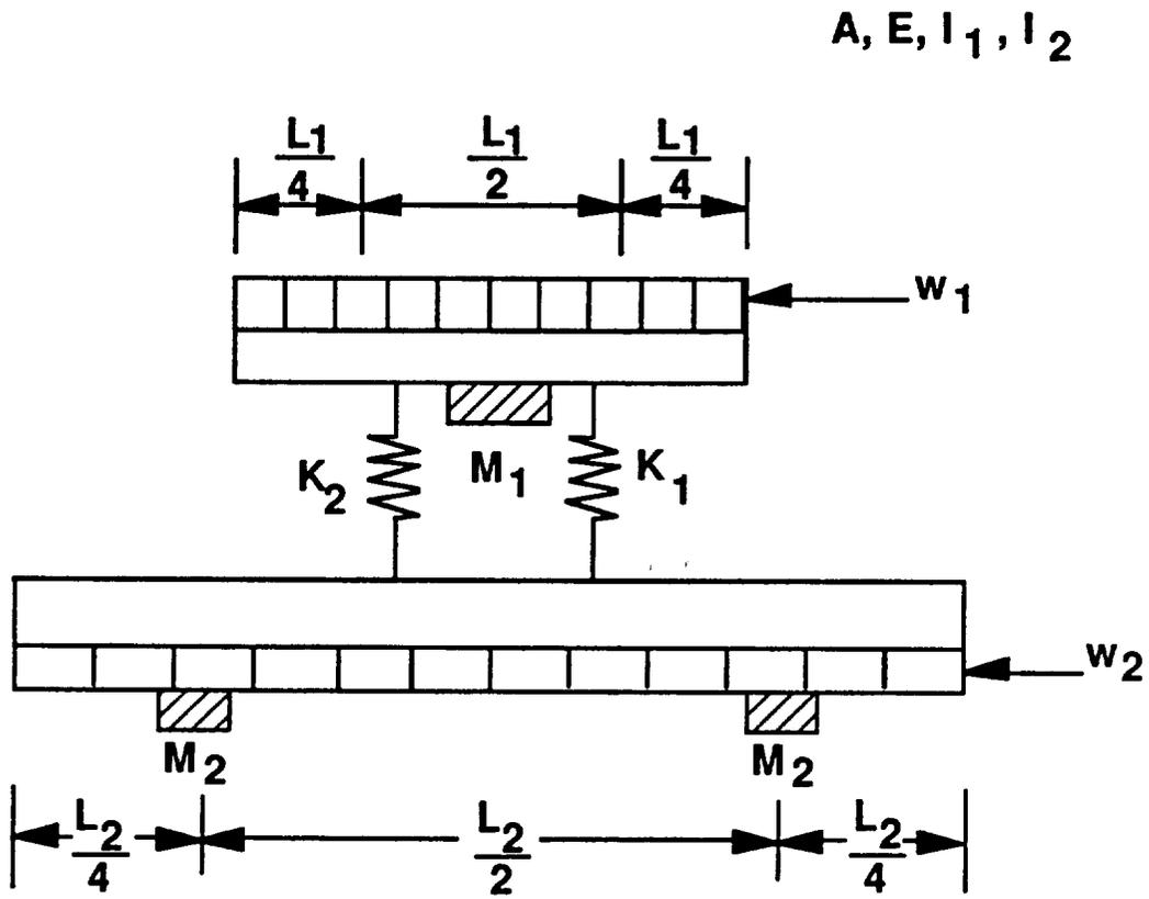
Figure 10. Two Beams Connected by Two Springs (Example 7)
