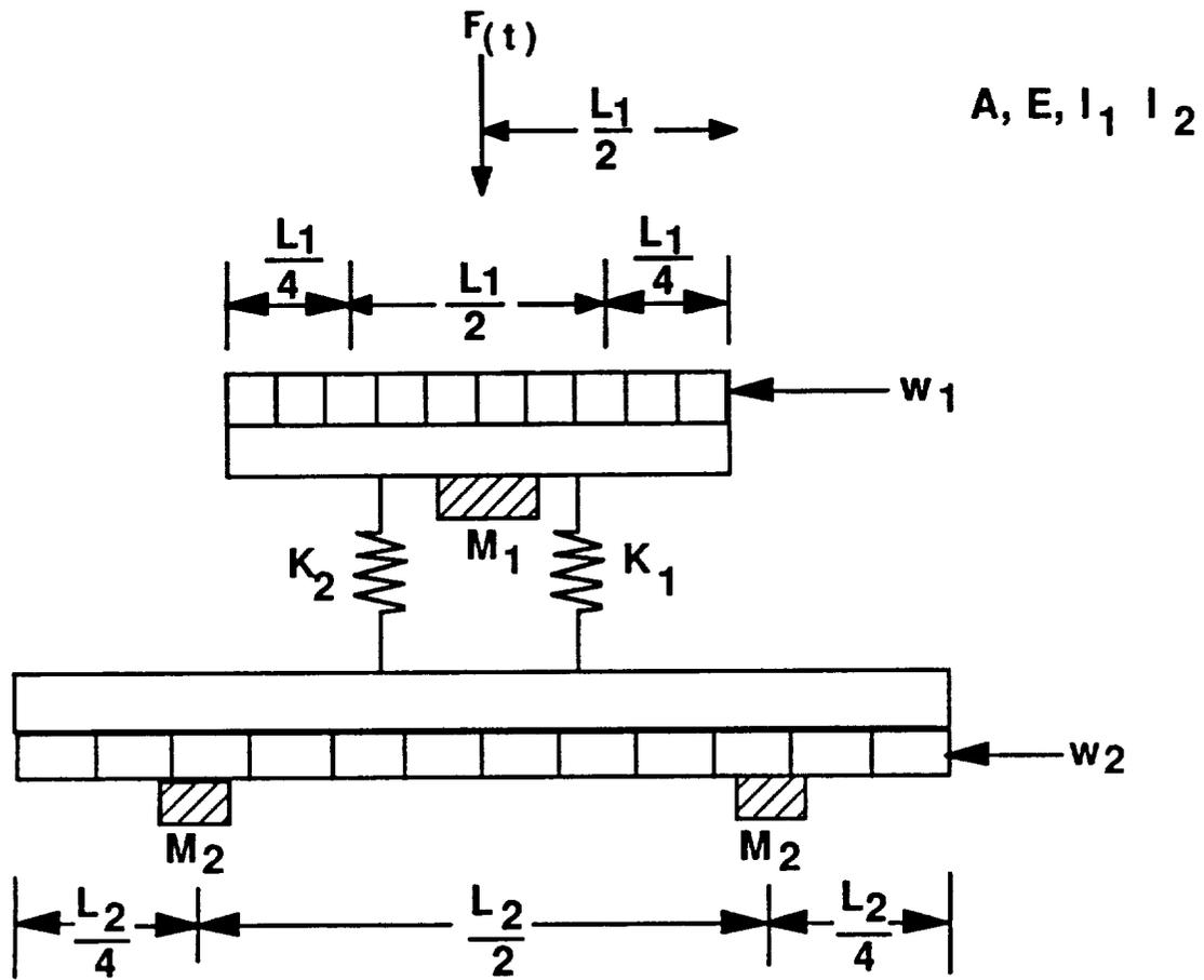
Figure 11. Two Beams Connected by Two Springs Driven by a Forcing Function (Example 8)
