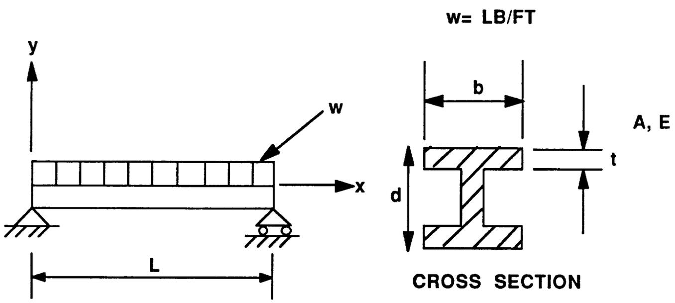
Figure 5. Simply Supported Beam with Uniformly Distributed Mass (Example 2)
