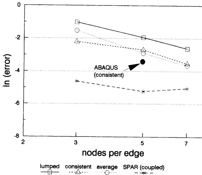
Figure 4. Frequency convergence for mode 3 of a flat plate as a function of mesh density for different finite elements.
