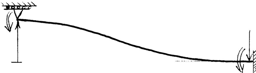
Note that the length remains invariant, because its transversely deformed end is not constrained in the axial direction. In effect, with this B.E. approach, the end position contracts when
