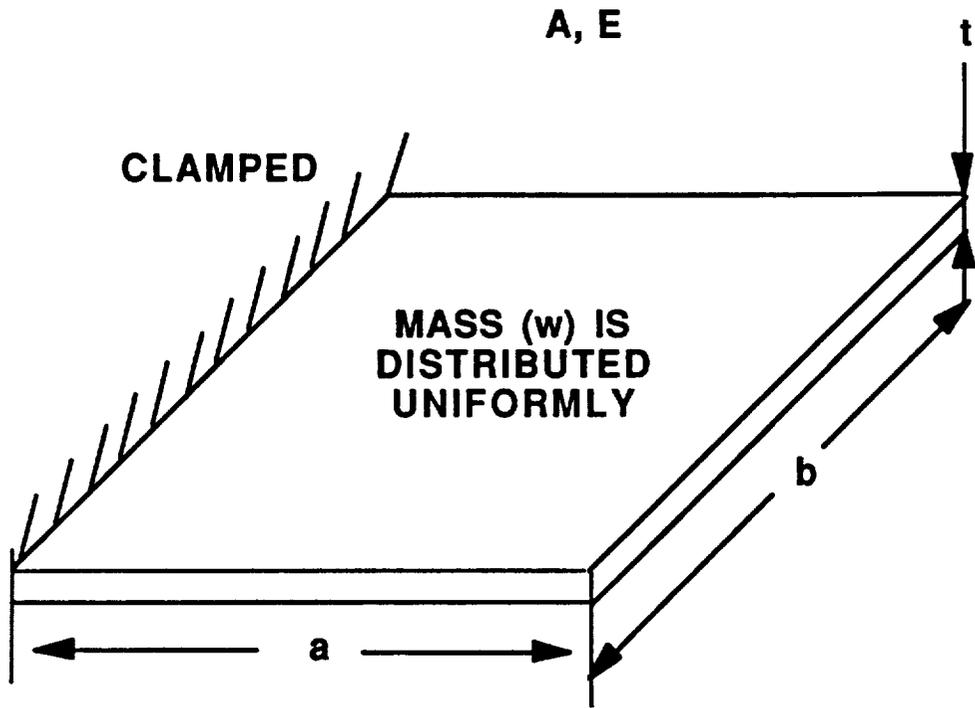
Figure 8. Rectangular Plated Clamped at One Edge (Example 5)
