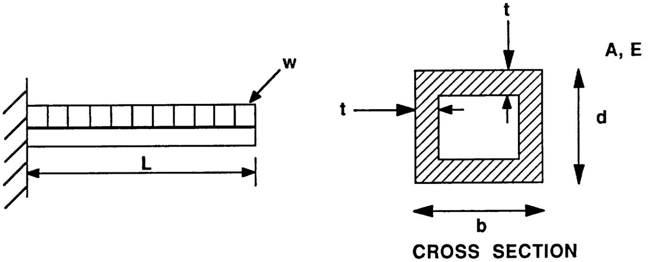
Figure 7. Cantilever Beam with Uniformly Distributed Mass (Example 4)
