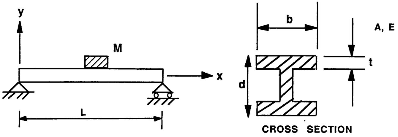
Figure 4. Simply Supported Beam with Concentrated Mass (Example 1)
