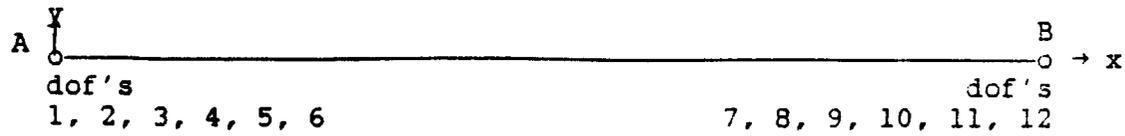
$$v_2 = 1 - 3\left(\frac{x}{L}\right)^2 + 2\left(\frac{x}{L}\right)^3$$
