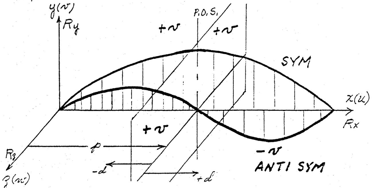
The elastic actions in XY bending require for symmetry that  $v(p-d) = v(p+d)$ . In the limit as corresponding points approach the p.o.s.
