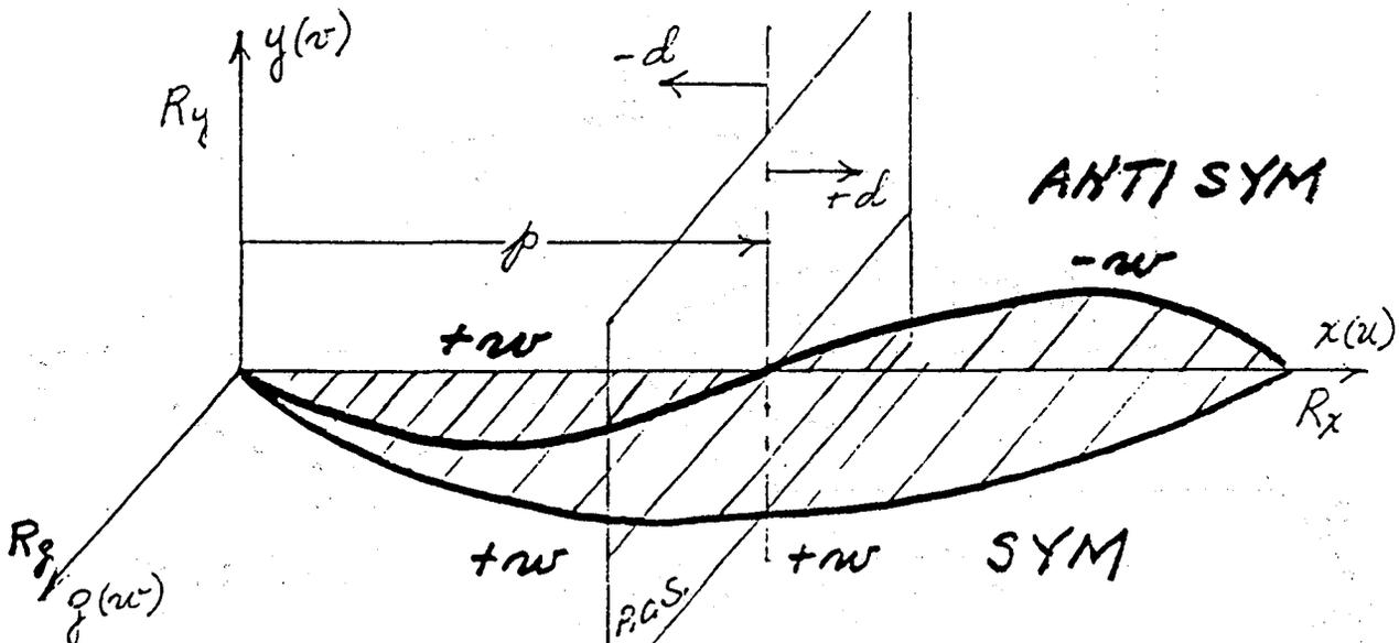
The elastic actions in XZ bending require for symmetry that  $w(p-d) = w(p+d)$ . In the limit as corresponding points approach the p.o.s.
