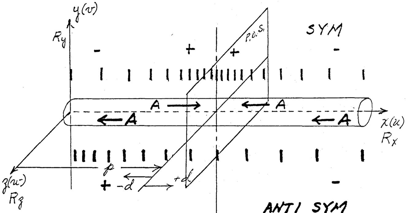
The longitudinal actions in X require for symmetry that both sides be either in condensation or in rarefaction; therefore axial forces, A, are equal and opposite
