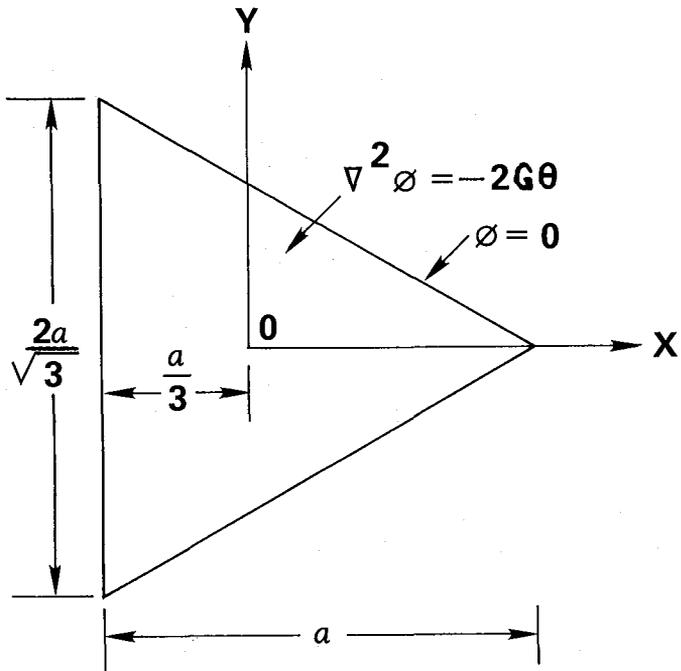
Figure 1 - Torsion of Triangular Prism
