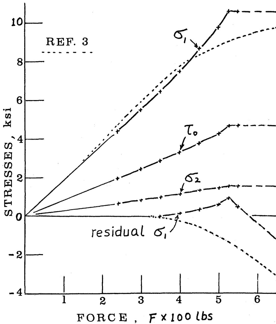
Figure 4. Stresses in Element 155 as Functions of Contact Force.
