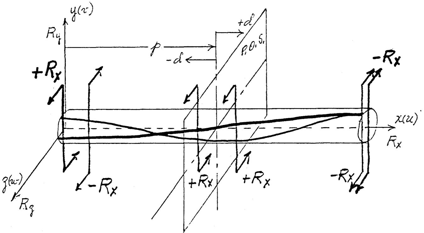
The torsional actions about X for symmetry require that  $R_x(p-d) = R_x(p+d)$ . In the limit as corresponding points approach the p.o.s.
