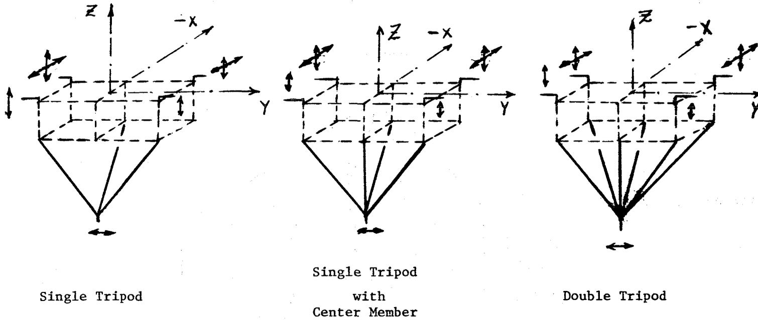
Figure 2. GAS Bottom Support Structures for Six-Pack Across-the-Bay Configuration.
