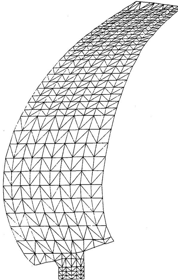
FIGURE 2 TURBOPROP PROPELLER FINITE ELEMENT MODEL
