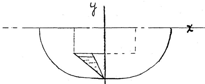
The case for the response in quadrant 1 can be stated in terms of reflections from quadrant 4 or from quadrant 2. The same results are obtained in either case. Referring to the signed tabulation for quadrant 4, the results for quadrant 1 become, as a result of reflecting the signed quantities of quadrant 4 about the X axis
