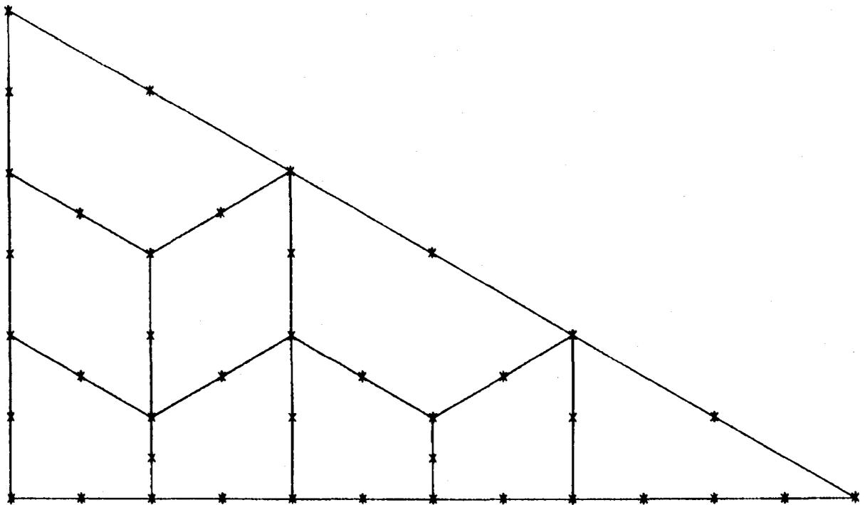
Figure 2 - Finite Element Mesh for Triangular Cross Section
