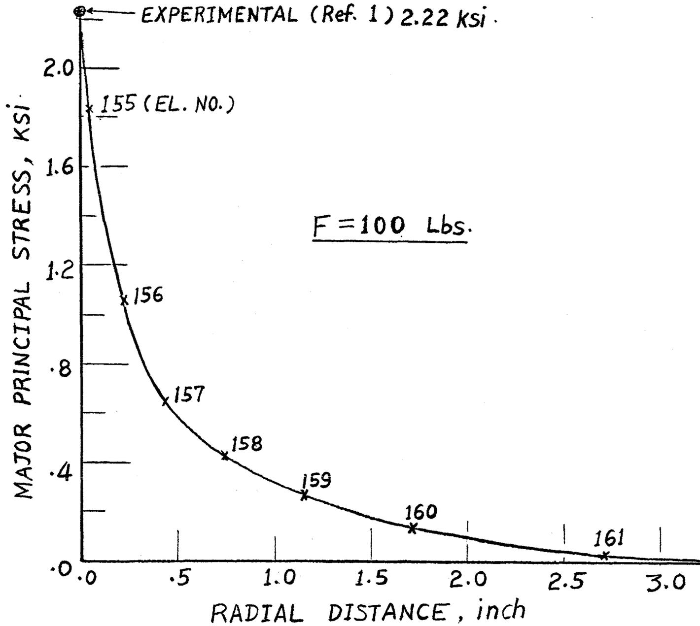
Figure 2. Maximum Tensile Stress for Elastic Loading.
