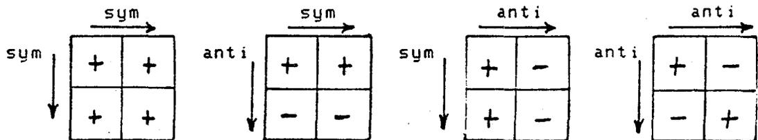
Let quadrant one be the model-quadrant. Four ingredient cases are constructed from the model quadrant with the 4 combinations of boundary conditions and each is given the same nominal load  $N$ .
