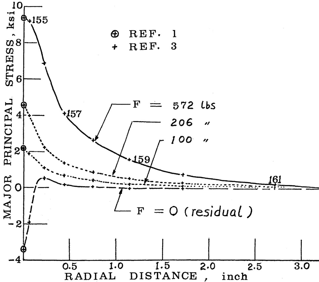
Figure 5. Determination of the Maximum Fillet Stress.
