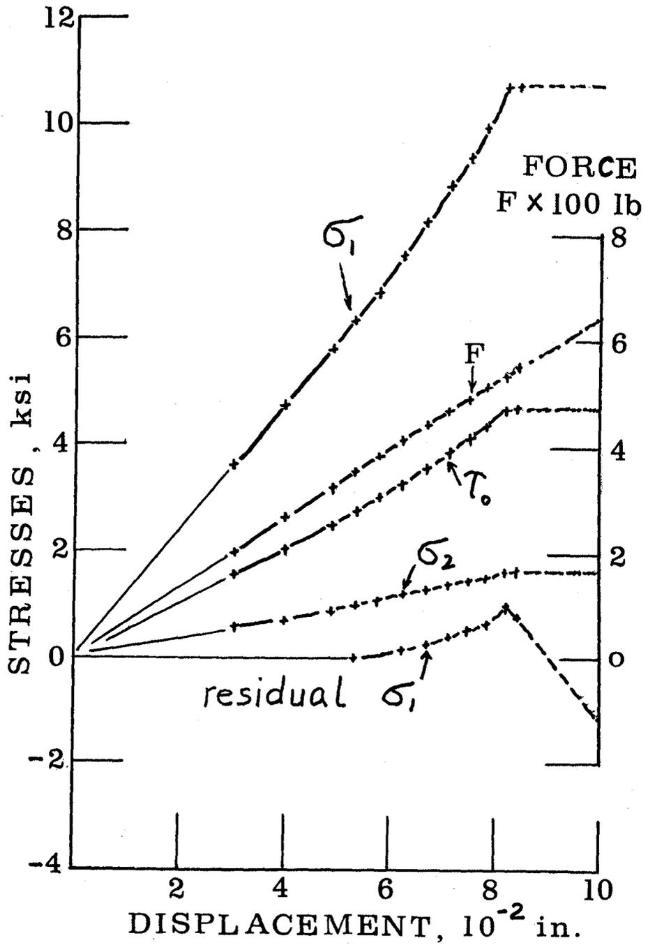
Figure 3. Stresses in Element 155 as Functions of Contact Displacement.
