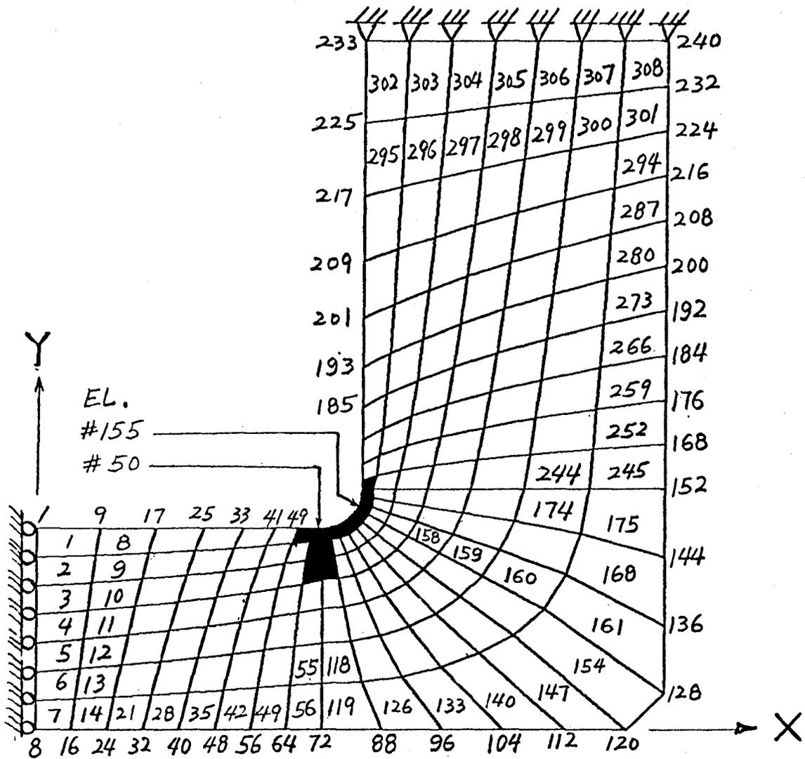
Figure 1. Finite Element Model for Breech Ring.
