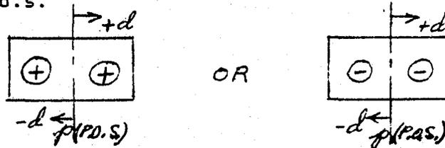
Antisymmetry maps the elastic deformations on one side of the p.o.s. into like values -- but of opposite sign -- on the opposite side of the p.o.s. at corresponding distances perpendicular to the p.o.s.
